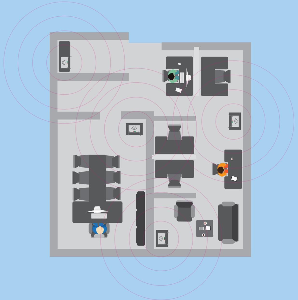
Channel utilisation and neighbouring channel interference within the coverage area needs to be assessed to determine what the optimal wireless frequencies are.
